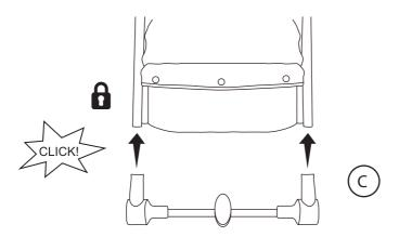
4. Connect the rear wheels (D) to the rear wheel axle. Push the wheel into the allocated area for the rear wheel, you will hear a "click" when secure.
